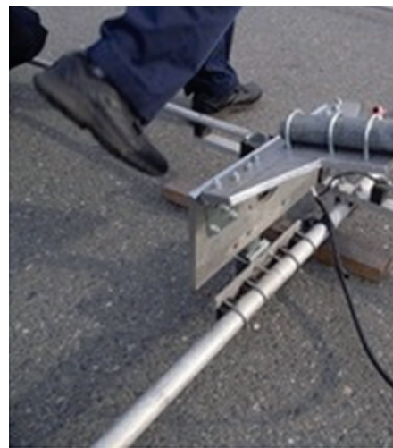
Let gravity be your friend by using this hinged Yagi mount designed by KL7VIC. (Photo by KL7RA)
