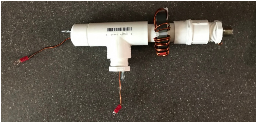
Figure 7: 40M Half-Square antenna mount with integrated Common Mode Choke
