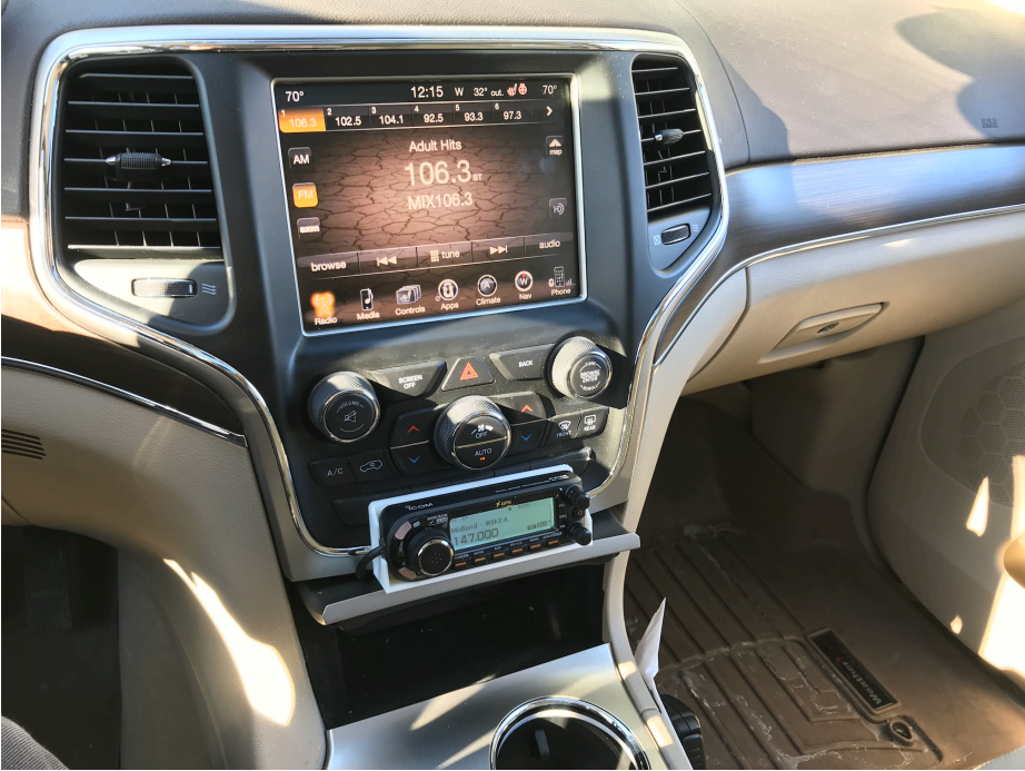
Custom bracket for Icom ID-4100 head
