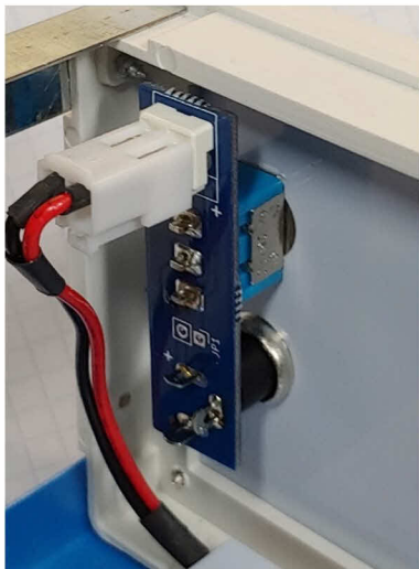
Power connector and switch after installation.
