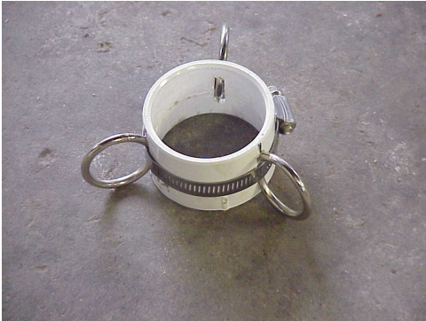
Completed upper guy ring
