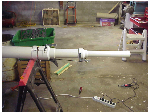
Final assembly of the reducers/pulleys and lift rope
