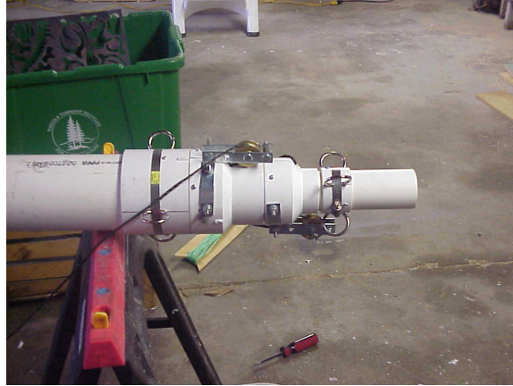
Upper guy ring mounted to final assembly
