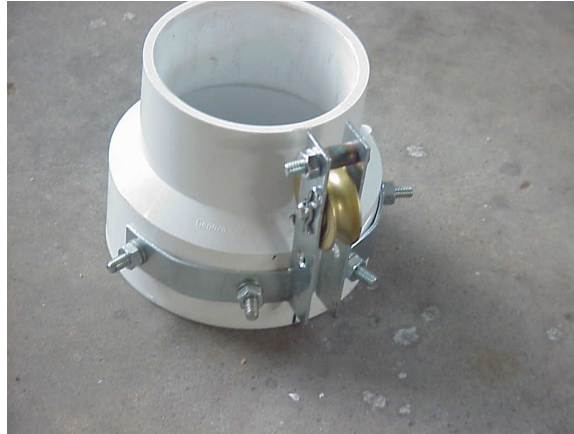
Finished upper pulley assembly
