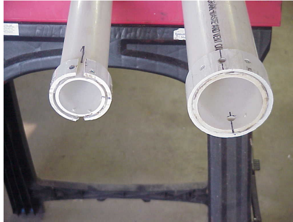
Lower guides mounted on the 2-inch and 3-inch pipes
