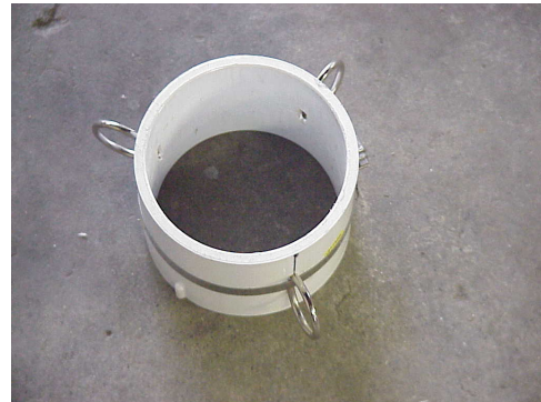
Completed lower guy ring
